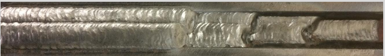
DW-50, 0.045", vertical upward welding at 64kJ/in with mixed gas
