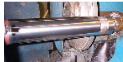
Forklift truck hydraulic ram, previously hard chromed, now coated with JK®120H. As sprayed (top) and during surface finishing (bottom) to 7 μ-inches (0.018μm).
